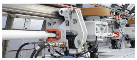
Friction wheels are the mostly used means of power transmission
