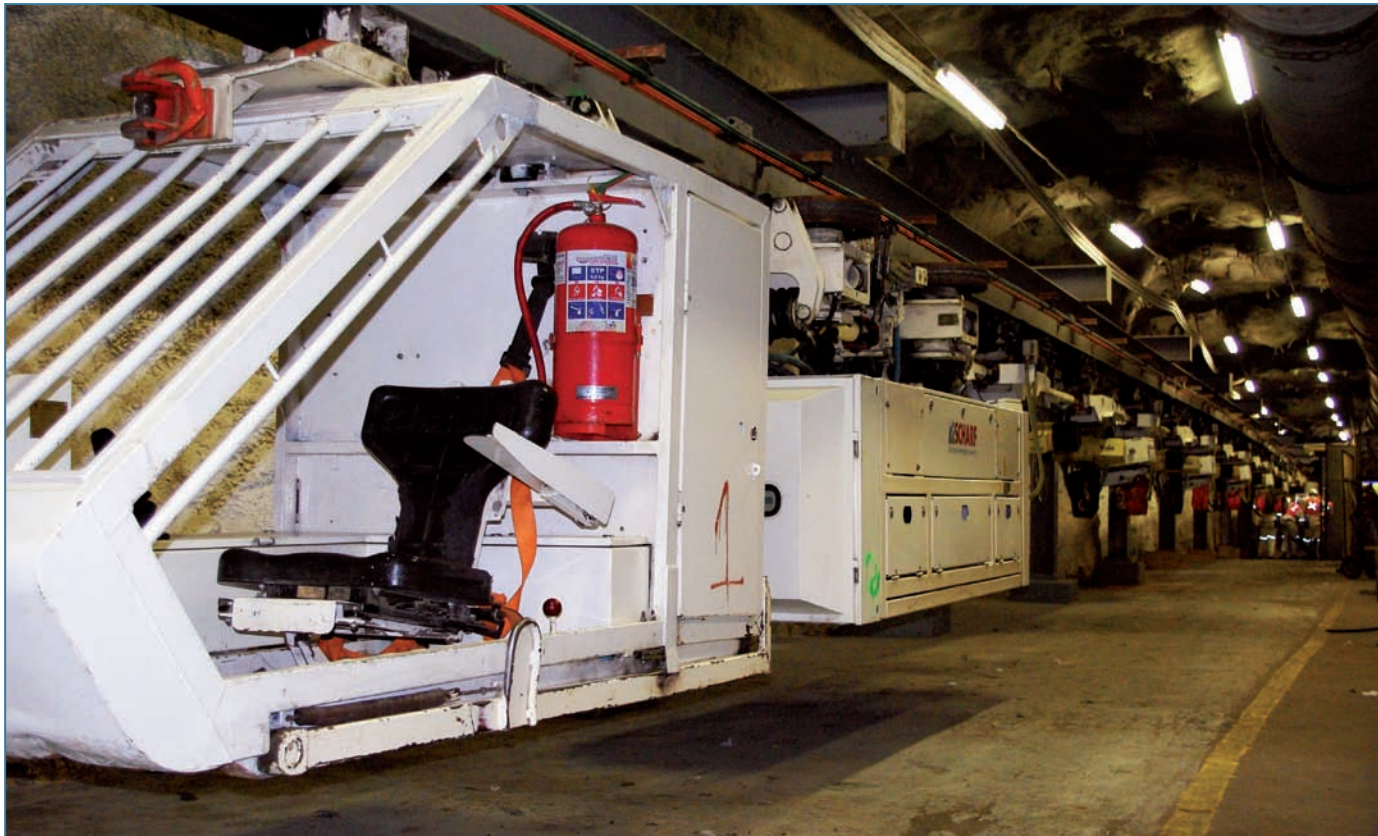
Electro-mechanical rail-bound railway system (EMTS)
