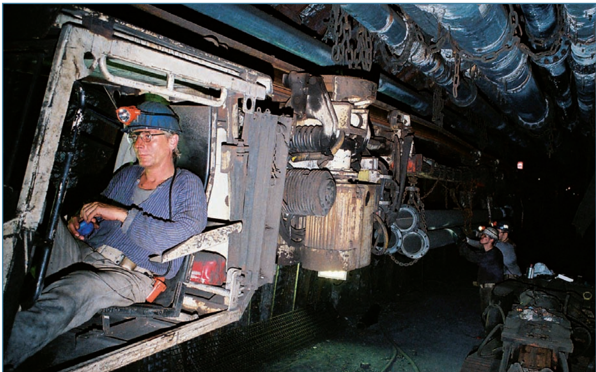
Battery-powered "cat" in the Ibbenbüren mine
