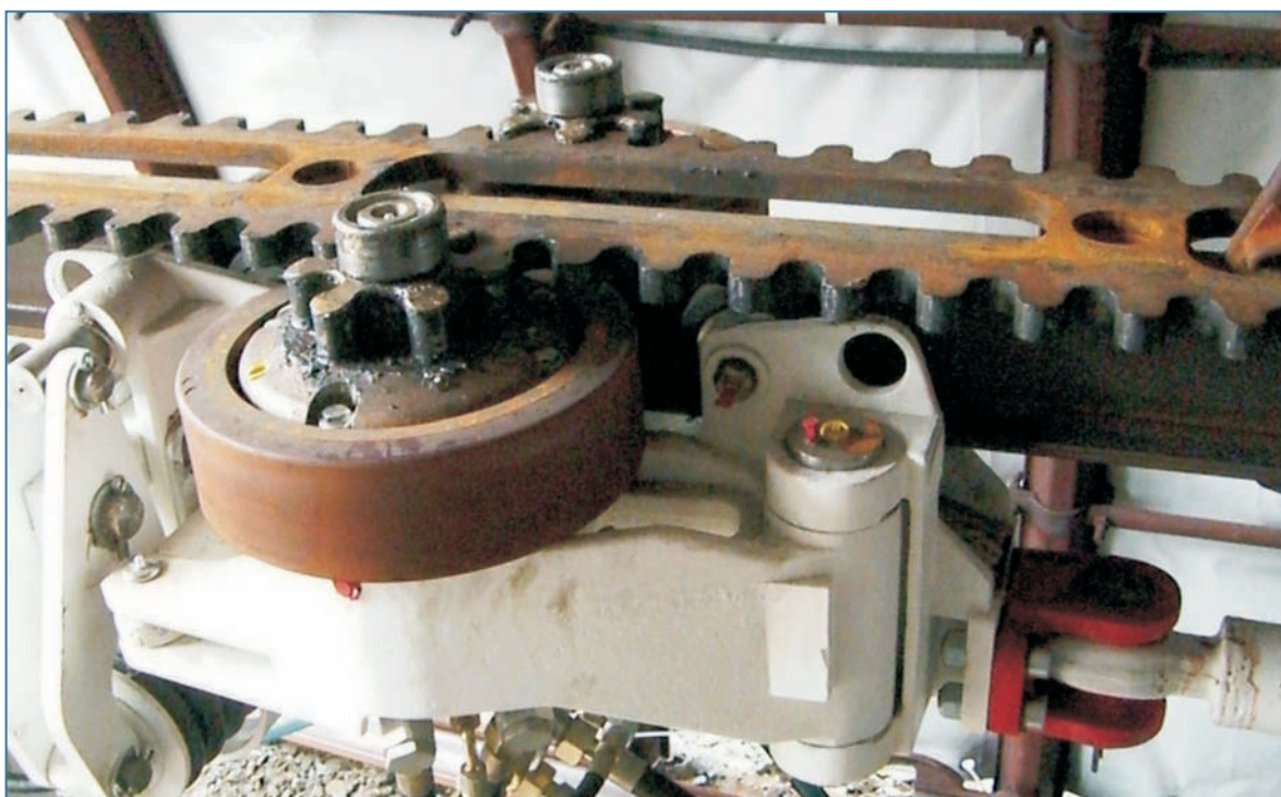
Switchable rack-and-pinion drive
